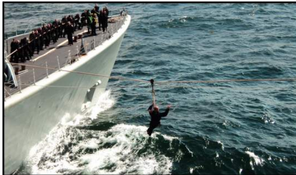
Task group patients transfer via helo, small boat and occasionally across a light jackstay as pictured here. It takes quite an ache to justify this dangling transit. Photo courtesy of Sgt R. Ross. Aug 2013.
